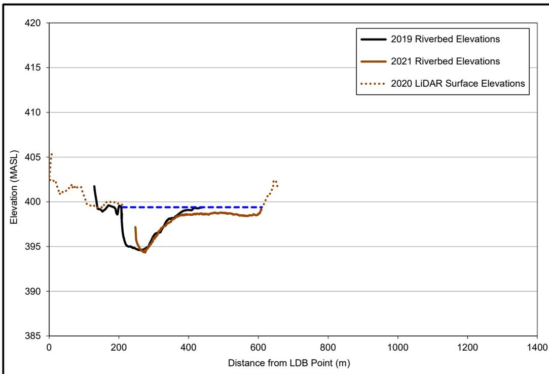
Figure B38: River cross-section at Transect #DS22, Peace River Physical Habitat Monitoring Program (Mon-3), 2021. The blue dotted line denotes water levels at the time of the 2021 survey. The channel differences are attributed to a survey misalignment in the field in 2019.
