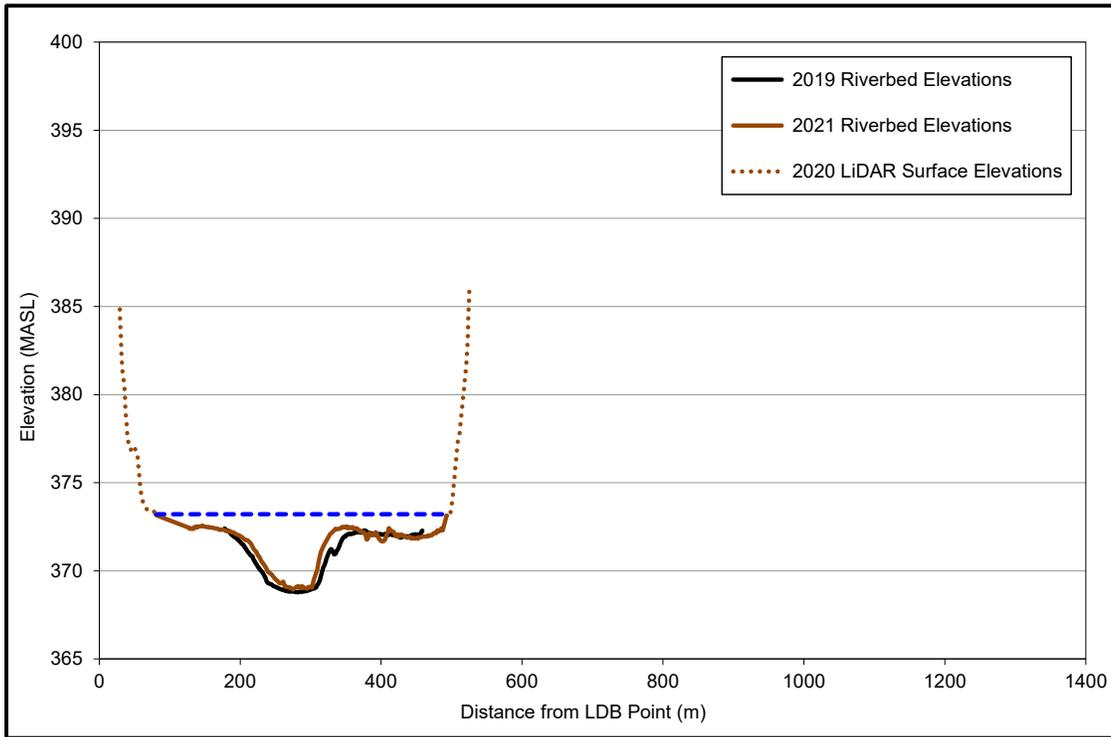
**Figure B49: River cross-section at Transect #DS33, Peace River Physical Habitat Monitoring Program (Mon-3), 2021.** The blue dotted line denotes water levels at the time of the 2021 survey. The channel differences are attributed to a survey misalignment in the field in 2019.
