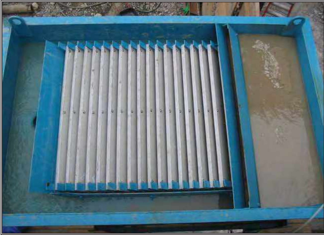
Inclined Plate Clarifier Tank commonly used for construction dewatering sediment removal.
