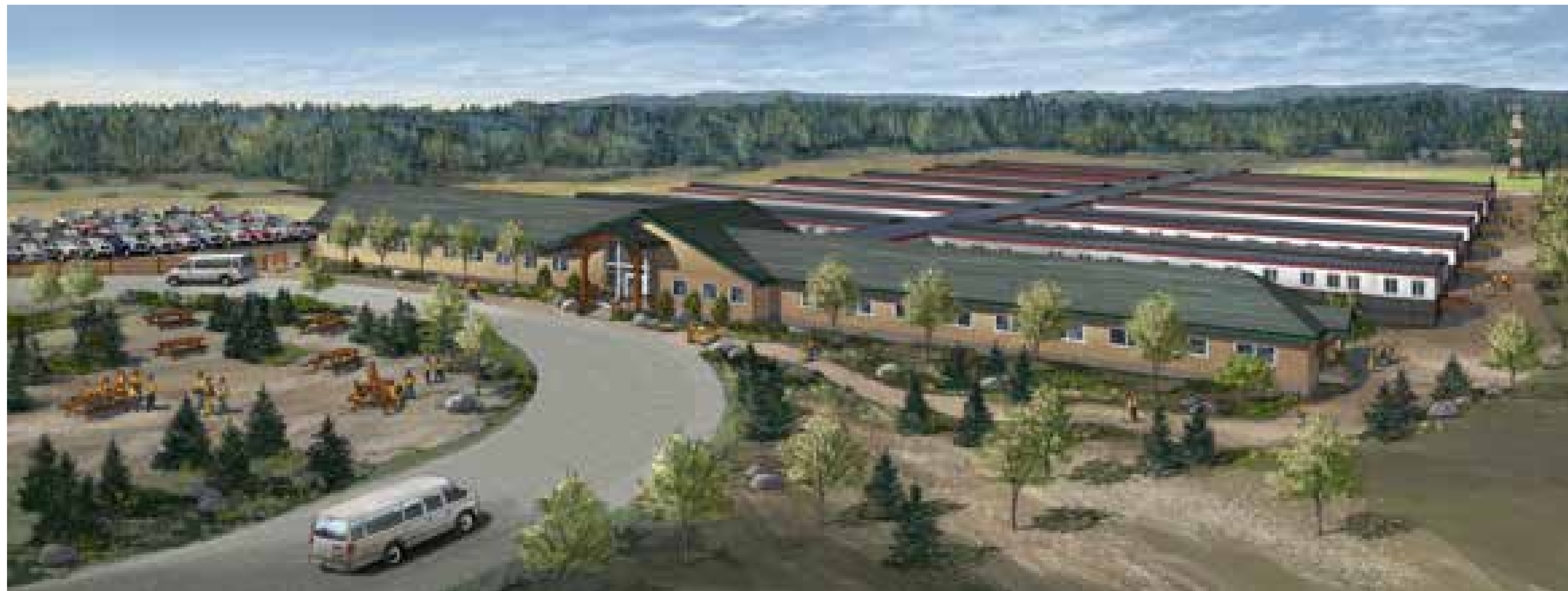
Artist's conceptual rendering of worker accommodation. This conceptual rendering shows modular units for approximately 500 workers, with a front lobby and common areas, transportation/shuttle loop, parking area, and rear dormitory wings accessible from a central interior corridor.
