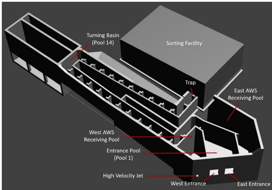
Figure 2. A drawing of the temporary upstream fish passage facility (TUF). Upstream migrating fish entered the fishway via one of the two entrance gates and ascended to the sorting facility for transport. Fishway attraction flows were provided by an auxiliary water supply (AWS) that flowed into receiving pools, into the entrance pool, and through entrances. A high velocity jet located adjacent to the fishway entrance provides supplemental attraction flow.
