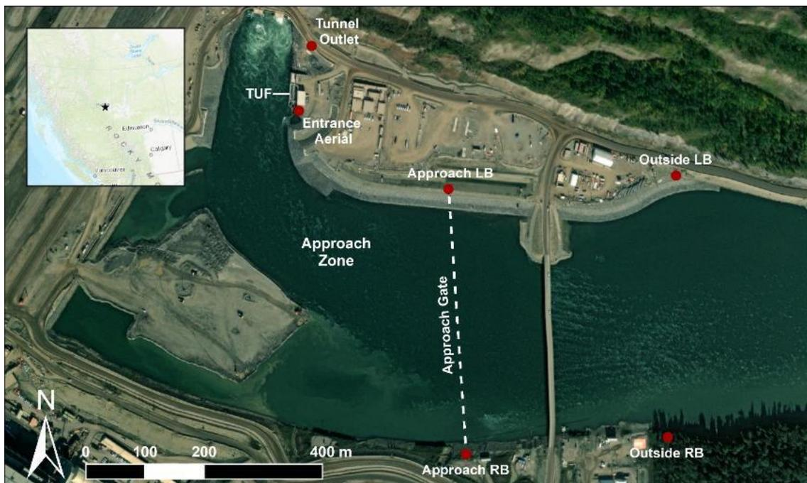
**Figure 3. The six aerial fixed radio telemetry stations deployed along the left bank (LB) and right bank (RB) of the mainstem Peace River and used to detect radio-tagged fish approaching the temporary upstream fish passage facility.**
