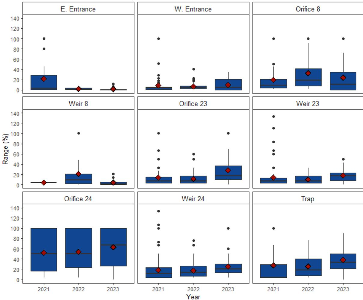
**Figure 11. PIT antenna test results using 32-mm HDX PIT tags, 2021 to 2023. Total read range (maximum distance a tag was detected) is presented as a percentage of the full read range (maximum possible distance a tag could be detected within, over, under, or by an antenna).**
