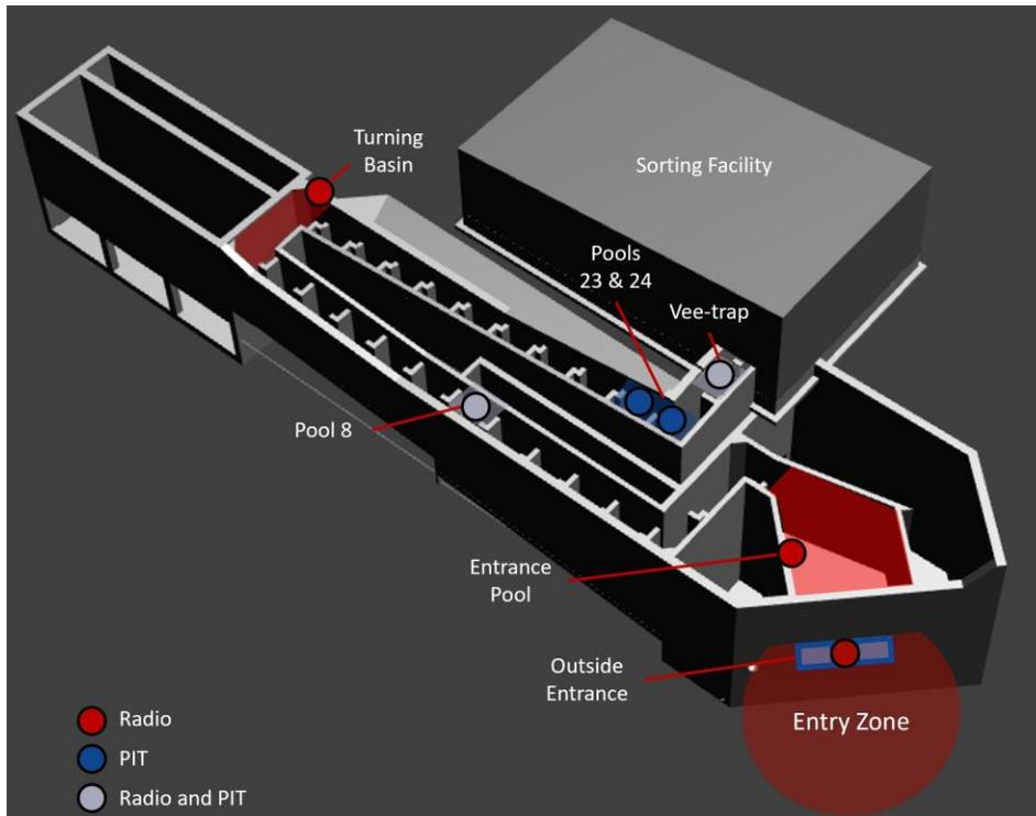
**Figure 4. Diagram of detection points via dipole fixed radio telemetry stations and passive integrated transponder (PIT) antennas within the temporary upstream fish passage facility. The target detection areas are shaded.**
