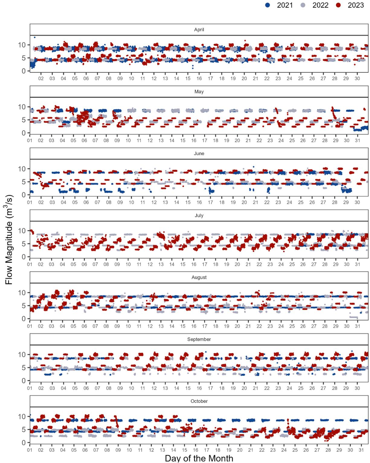
**Figure 7. Attraction flows from the auxiliary water supply recorded every 10 minutes from the temporary upstream fish passage facility during the operational period in 2021 (blue), 2022 (grey), and 2023 (red). Only data from when the fishway was operational is shown (i.e., shutdown periods are excluded). Data provided by BC Hydro.**
