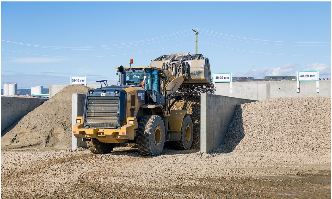
Photo: Aggregate materials, such as gravel, are produced and sorted on site.
