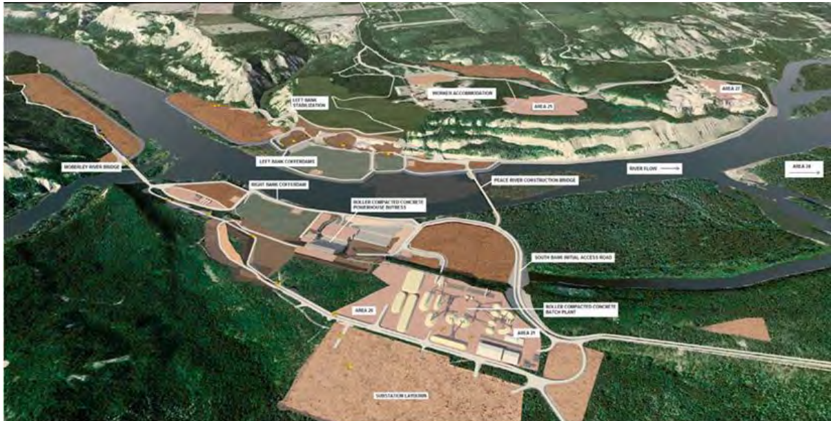
Figure 2 An Artist's Rendering Depicts the Site C Earthfill Dam, Generating Station and Spillways, Substation, Transmission Lines and Reservoir 8
