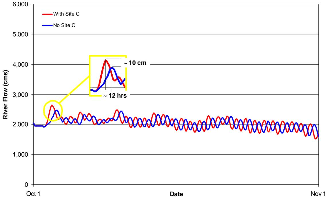
**NOTE:** Modelled flow is represented. Figure is based on an optimization model scenario for an average discharge year with constraints (i.e. min/max flows at Site C of 283 – 1,982 cms combined with the daily local inflows). Actual flows may vary based on load and operational constraints.
