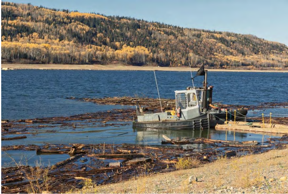
Figure A-1 The sidewinder boat is used to move logs and woody debris from the reservoir to the shoreline
