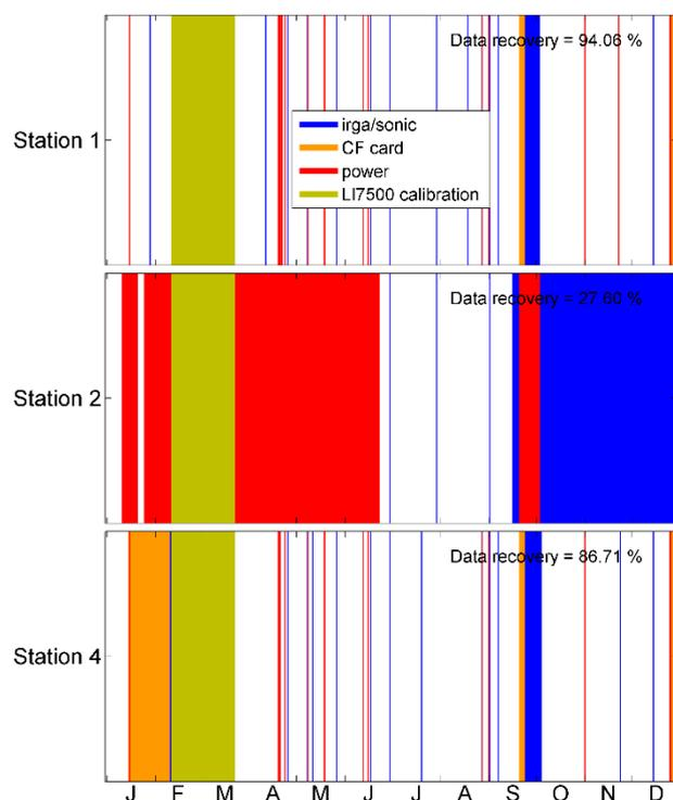
**Figure D1.** EC system performance for Stations 1, 2, 4 in 2016 indicating sources (IRGA/sonic anemometer failure, CF card malfunction, power (low battery voltage), IRGA calibration) of data loss prior to manual QA/QC of the data. Vertical bars indicate flux data loss. Annual data recovery percentage indicated in each panel.
