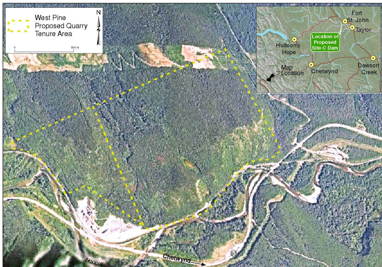
Figure 4.5 Potential Source of Construction Material at West Pine Quarry Near Pine Pass
