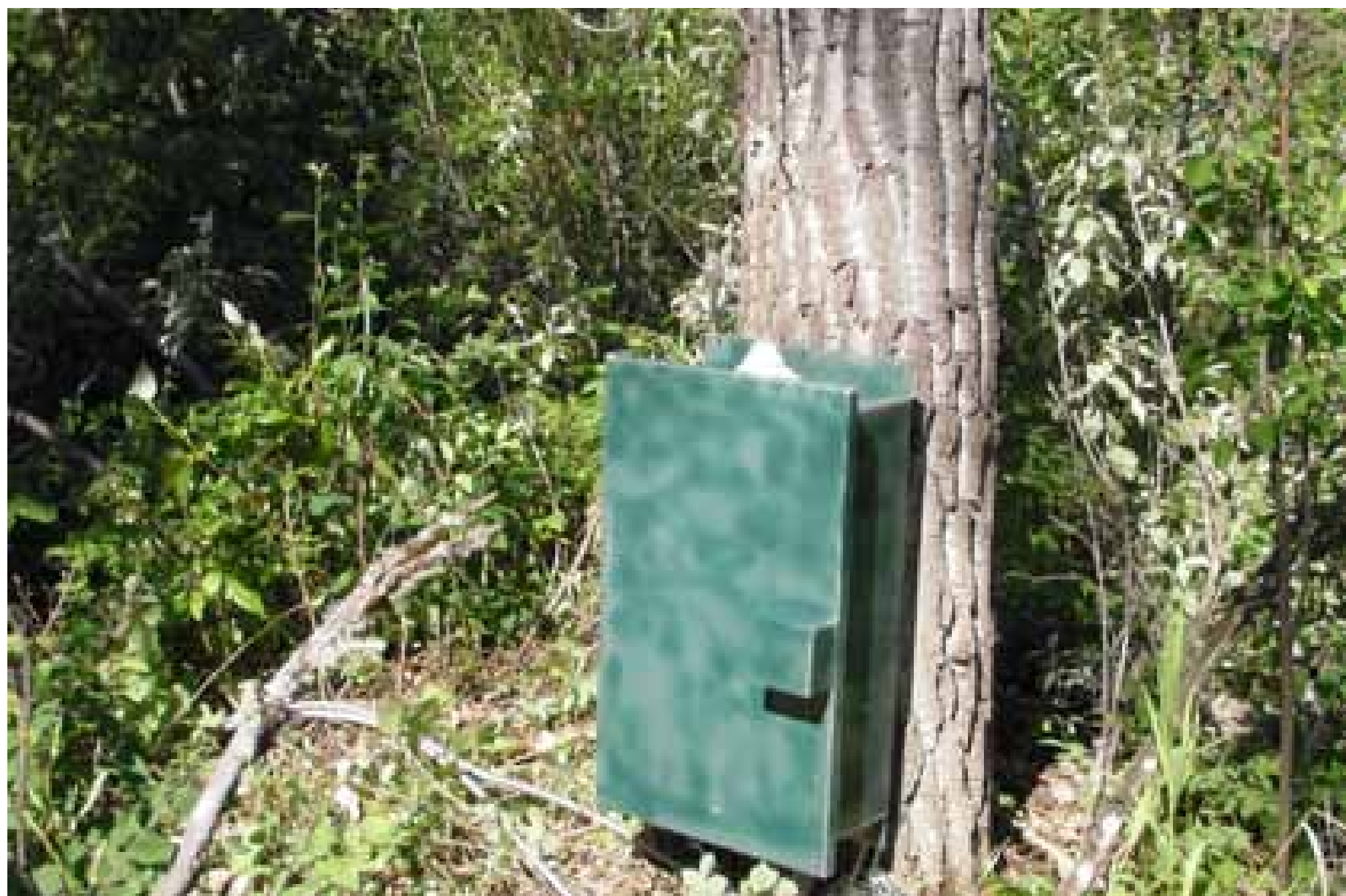
Turbidity sensor data logger housing
