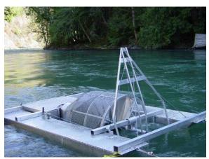
Photo of a rotary screw trap in operation
