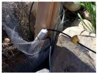
Photo 28: Installation of extra insulation to the tube housing hibernaculum temperature logger. Silicone sealant used to seal cap onto top of tube (11 June).
