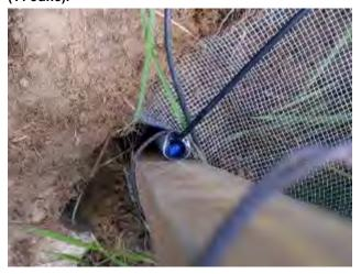
Photo 27: Installation of extra insulation into the tube housing hibernaculum temperature logger. Insulating foam inserted into tube (11 June).
