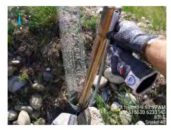
Photo 25: Example of procedure to install extra insulation to the tube housing hibernaculum temperature logger. Tube cut close to ground level (11 June).
