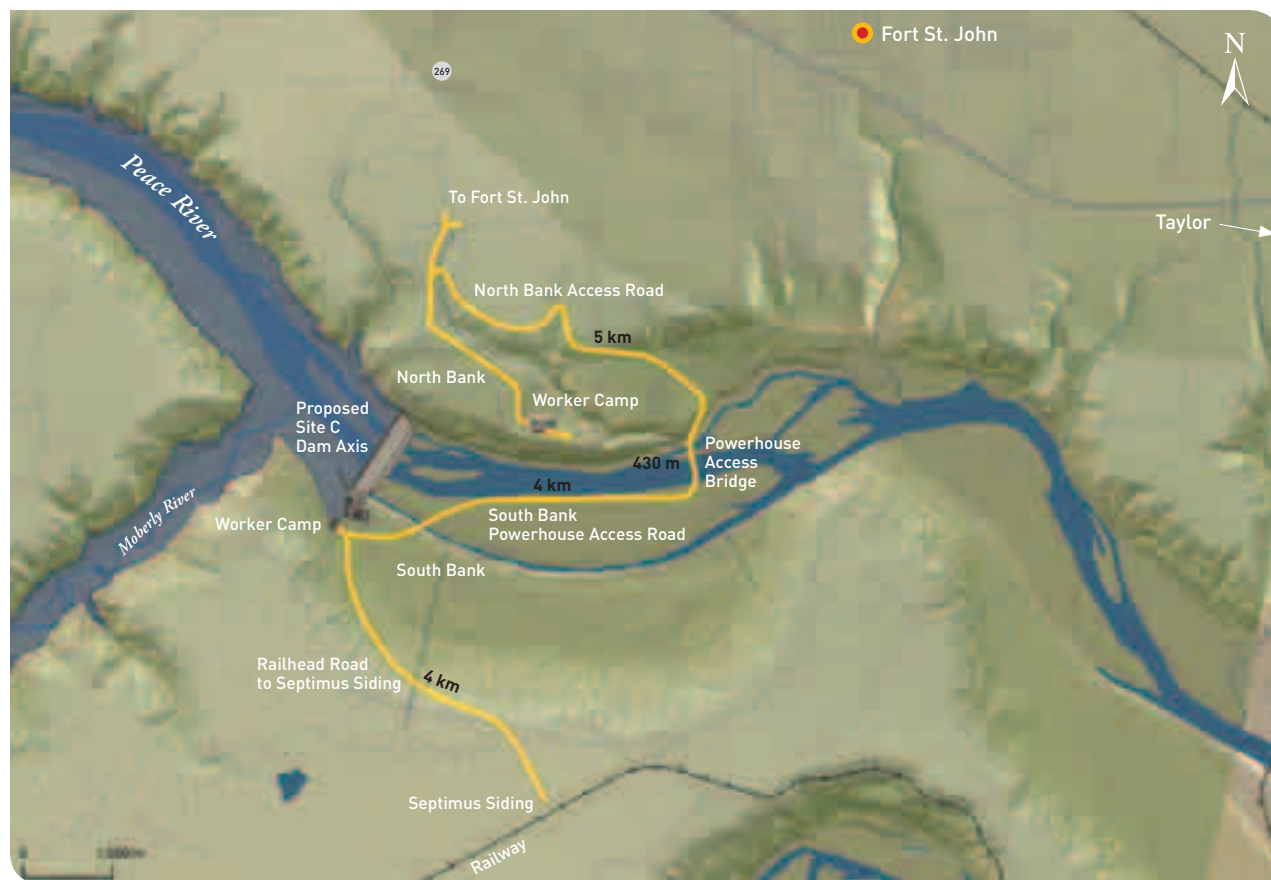
FIGURE 6-9: POWERHOUSE ACCESS AND PEACE RIVER CROSSING
