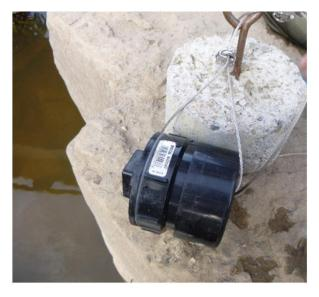
Figure 2: Examples of temperature logger housings deployed during the Site C Reservoir and Peace River Water Temperature Monitoring Program (Task 2b). The photo on the left denotes housings initially deployed during GMSWORKS-2. The photo on the right denotes housings initially deployed during Task 2b.
