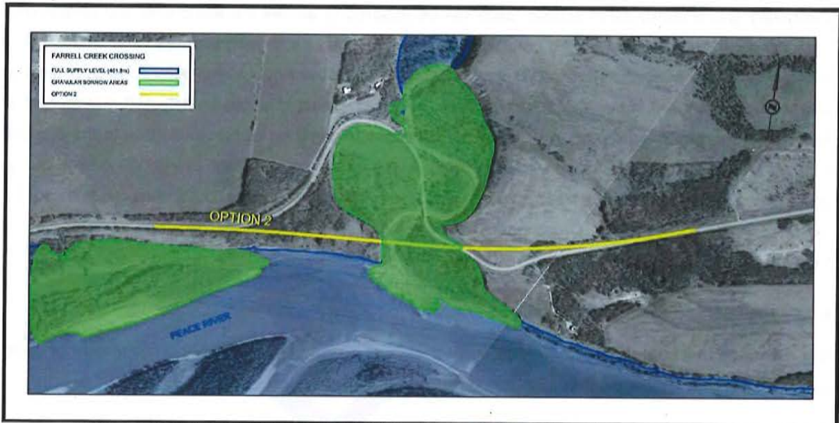
Figure 5.3.2: Potential Granular Borrow Sources at Farrell Creek
