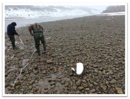
Plate 2 View downstream of interstitial transect sampling along a recently dewatered portion of a gravel bar within Reach 1 (October 14, 2016).
